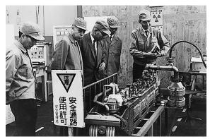
Figure 4. A prototype accelerating tube of 15-MeV Linac
