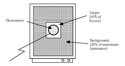
Figure 7 Test pattern and sensor placement example
