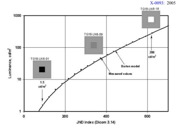
Figure 8 Example plotted by relating the luminance measurement values of 18-step display levels to the DICOM 3.14 standard luminance response
