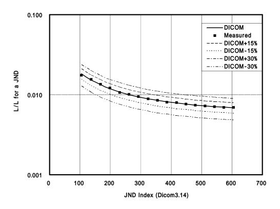
Figure 9 Example showing how the contrast response calculated from 18-step gray levels relate to the contrast expectation response relating to the DICOM3.14 standard contrast response
