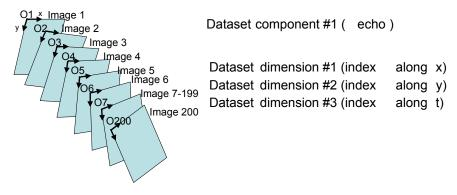
Origin: 200 Occurrences with x,y,z coordinates of O1,O2,..., O200, indexed by Dataset dimension #3 ¢orresponding to t1, t2,..., t200) Direction cosines: 400 Occurrences with 200 concerning Dataset dimension #1 (x)ndexed by Dataset dimension #3 (idem t1, t2,..., t200) and 200 concerning Dataset dimension #2 (y)ndexed by Dataset dimension #3 (idem t1, t2,..., t200)
